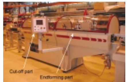
Chipless linear motor based tube cut-off with integrated endformer
