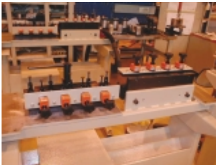
Quick changeable straightening rolls and digital readouts
